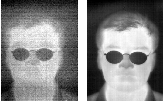
Figure 1: Calibrated (right) and uncalibrated LWIR images. There is significant pixel-wise difference in responsivity which is removed by the calibration process.
